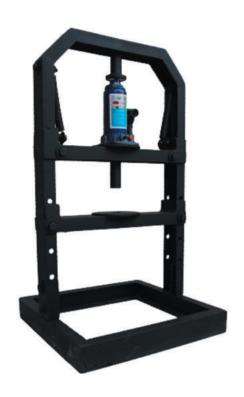
The heavy duty hydraulic puller from Kisan Engineering makes your job very easy. With the help of this puller, you can easily remove the shaft and bearing of any fan and motor. You can buy hydraulic puller from 10 ton to 20 ton as per your requirement. Due to the hydraulic puller heavy iron body of Kisan Engineering, you can do heavy work on our puller. You can get it anywhere in India.
