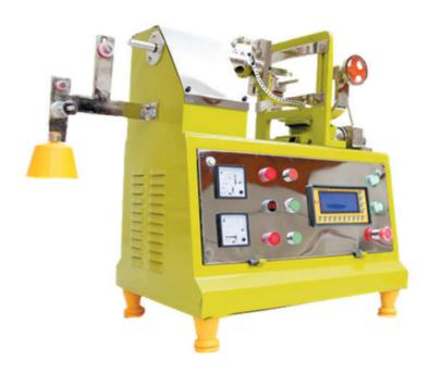
KIJ-125 is a modern model manufactured by Kisan Engineering. In this machine you can make coil from 1 hp to 10 hp along with ceiling fan winding. There are 2 turns in this machine. 1. Fan Winding 2. Coil Making
